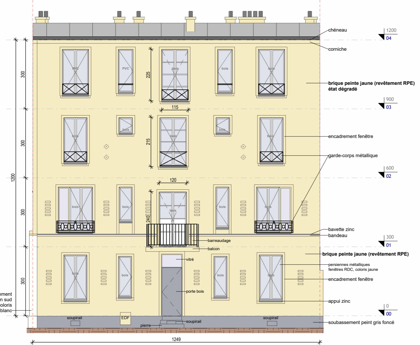
FACADE RUE EXISTANT
